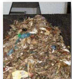
The separated contraries are mainly plastics, wood parts but also textiles and light metal foils. This material is delivered as RDF to a power plant. The heavy fraction, containing the stones, glass, porcelain, bones and metals, must be disposed to a dump side.
